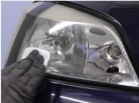
Repeat this process as many times as necessary until the light/tail light is visually clear. (Usually 2-3 times.) Remove all residues that remains by polishing dry.
